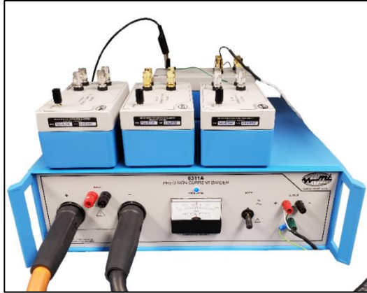
Figure 4. A Measurements International 6311A Precision Current Divider (or DCCT) and four standard resistors
