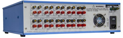
The resistor elements mounted in the chamber are the same elements that are used in the MI 9331 series of standard air resistors. The temperature coefficient of these resistors is reduced by controlling the temperature of the internal chamber to achieve its excellent long term stability.
