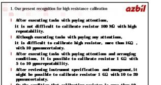
$\mid$  On the condition that calibrating resistor is more than 10 GQ, the task needs many attentions and it is not easy to judge the resistance value adequate one. The information for standard resistor is poor.
